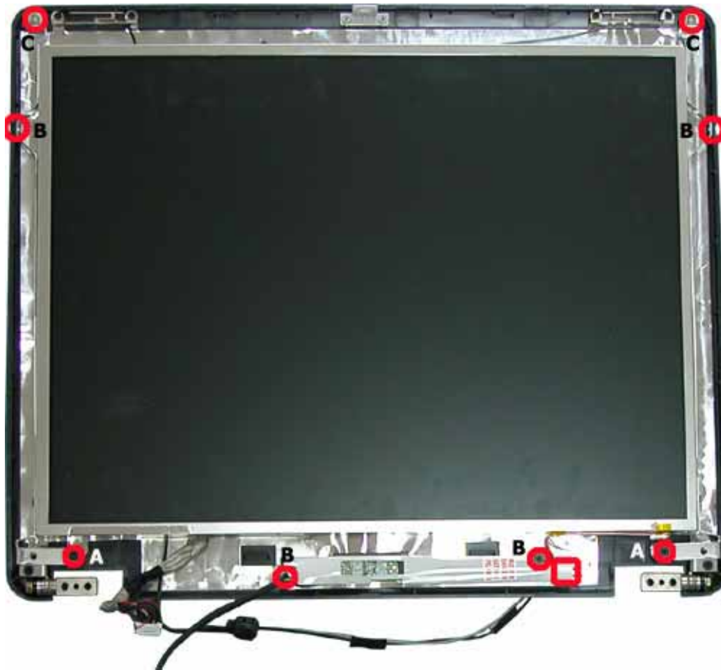
Fig. 27 Removing the LCD panel screws
